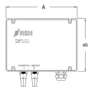
The CLE boards are pre-wired tested and ready to be installed on board, they are used to manage the solenoid valves, the pumps and the various control inputs. They range from the simplest to those equipped with an electronic controller (PLC).
